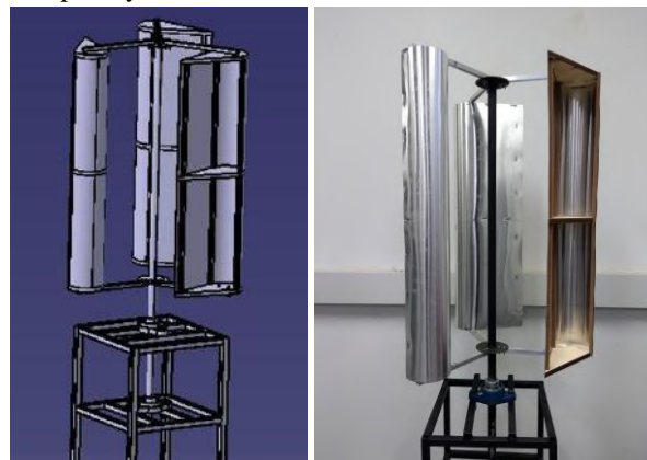
Fig. 8: 3D-drawing and photo of the Lenz-type VAWT.
