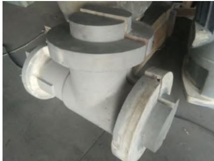
Fig.11: Wooden pattern middle part ESV
