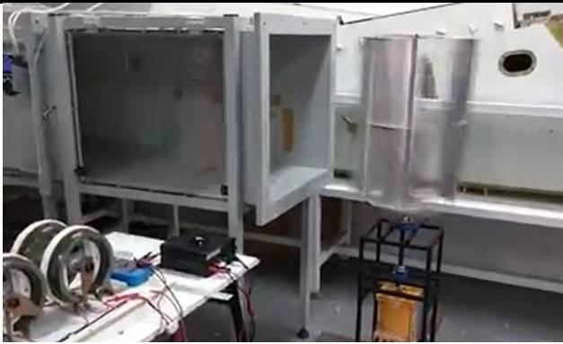
Fig. 9: Lenz-type turbine under tests.
