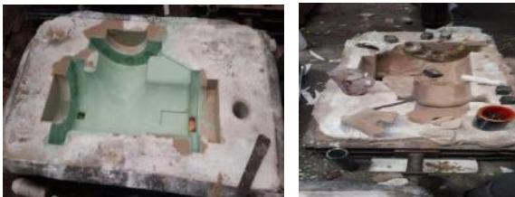
Fig.12: Mould box middle part ESV
